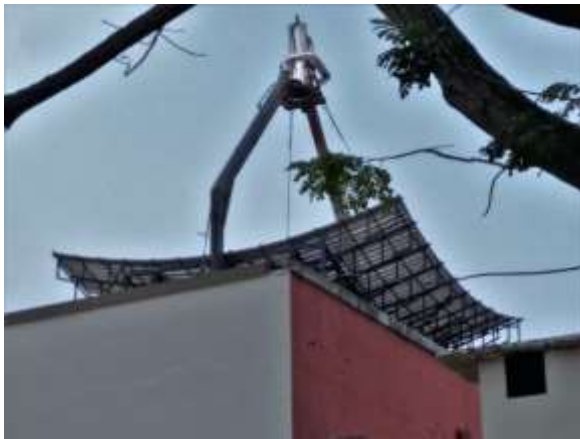
Fig.17 CSP* Concentrated Solar thermal for power generation (ABD,TNAU,CBE-Dual axis tracking installation)( ABD-TNAU coimbatore : Dual axis tracking of sun's movement
