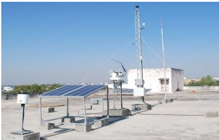
Fig.4 Sensors of a typical SRRA station
